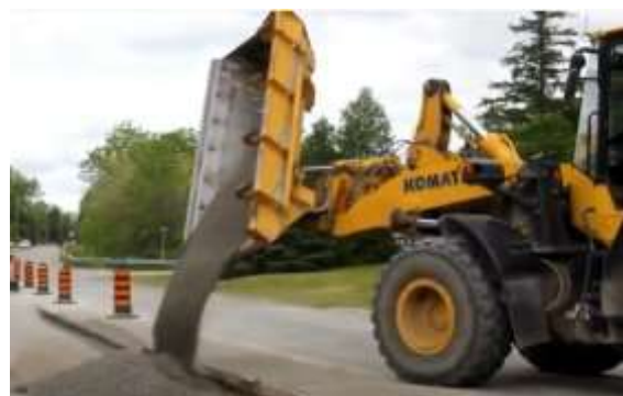
Figure 1. Work principle of loader with side discharge bucket.
