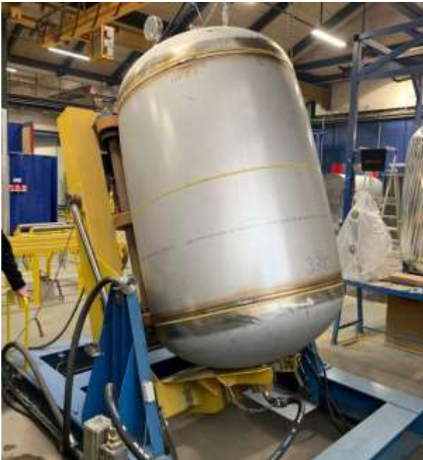
Figure 8: The cold stretching installation and the tank
