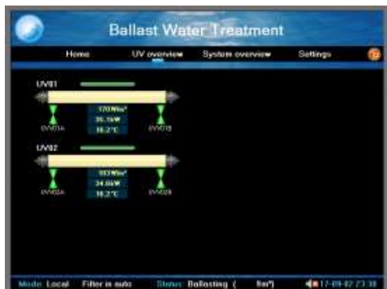
Figure 9: UV-lamps Monitoring, UV-radiation, electrical power, temperature [6].
