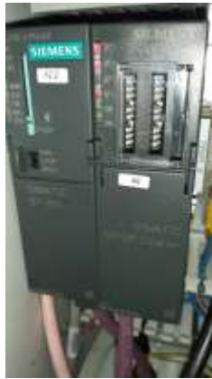
Figure 5: A Model of a PLC-type Programmable Controller [6].
