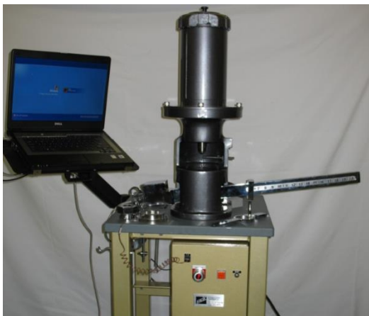
Figure 1: Falex testing equipment [Falex]
