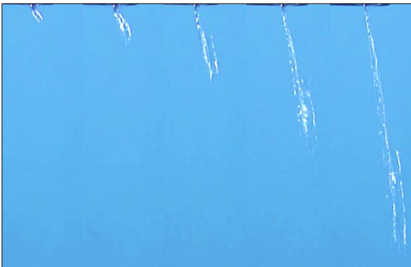
Figure 8: Presentation in five stages of the evolution of the atomized fuel jet at the studied injector.
