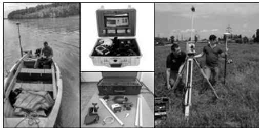
Figure 3: Single beam sonar for depth measurements, RTK GNSS linked with sonar and total station for bank points measurement
