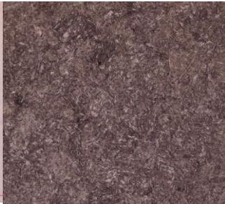
Figure 4. Etched microstructure of bolt #7 on the core, 200X
