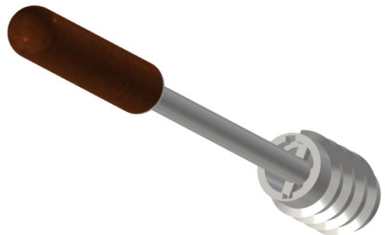
Figure 52: The assembly tool inserted in the T-slot of the threaded component. In this way the threaded component is screwed and unscrewed in femur.
