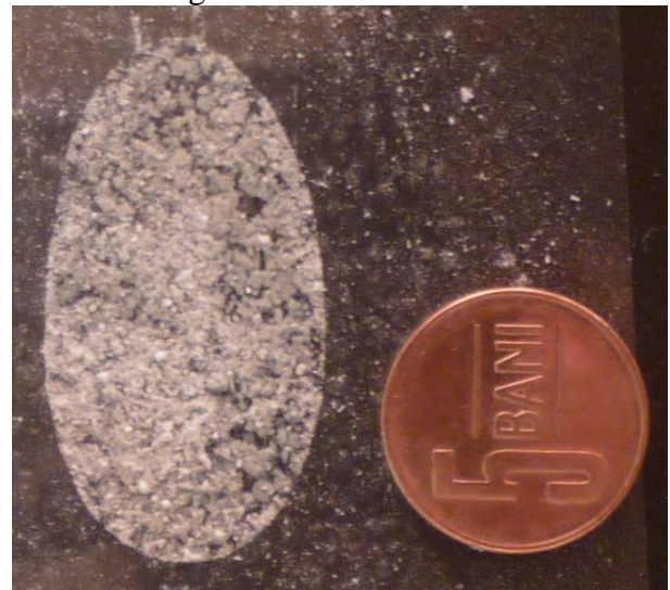
Figure 2: Example of the lubricant trace. Gears oil, roll steel/porous layer, v=3.4 m/s.
