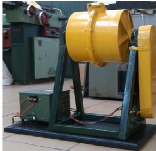
Figure 1: Equipment for grinding metal waste (Ball mill); scheme of the ball mill: 1 – Mill bed, 2 – Frame, 3 - Bearing cover, 4 – Bearing, 5 - Bearing Support, 6-10 - Drive shafts, 7 – Mill case, 8 - Cover, 9 – Admission hopper, 11-15 – Belt pulley, 12 – Case, 13 -Drive Belt, 14 – Motor, 16 - Motor shaft, 17 – Balls
