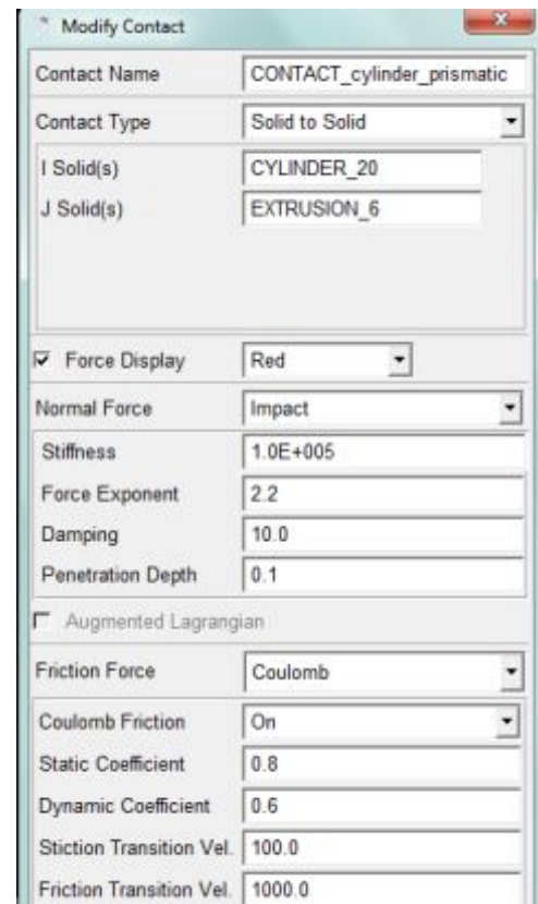
Figure 4: The dialog box from simulation software for friction parameters setting
