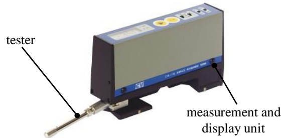
Figure 5: Portable surface roughness measuring device
