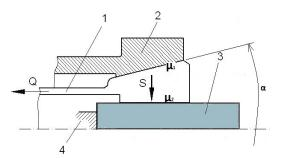
Figure 2. Physical model of request: 1-collet, 2-conialc sleeve, 3-study object, 4stopper
