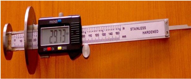
Figure 5. Digital device for internal conicity measurements
