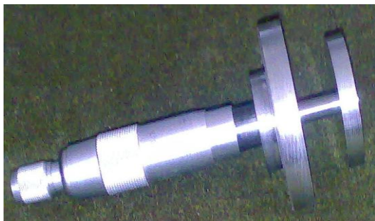
Figure 6. Micrometric device for internal conicity measurements
