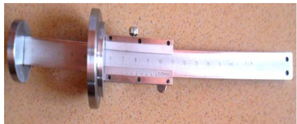
Figure 4. Vernier device for internal conicity measurement
