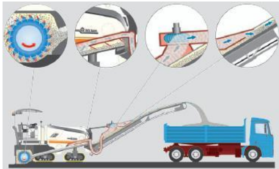
Figure 5: Cold recycler equipment with vacuum cutting system (Wirtgen Inc.)
