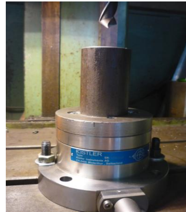
Figure 18: Sample reinforcing – adapter piece – dynamometer
