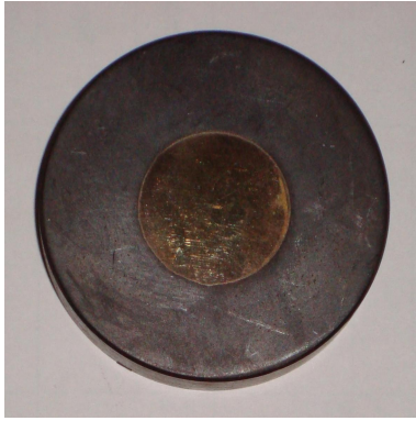
Figure 5: Good adherence of bronze on the steel surface for the bimetal sample obtained at 1300°C, slowly cooled with furnace (surface after exposure to metallographic attack)
