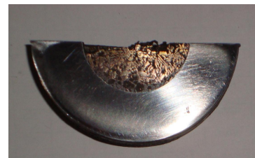
Figure 4: Bronze chips incomplete melted that were heated at 1200^\circ\text{C}
