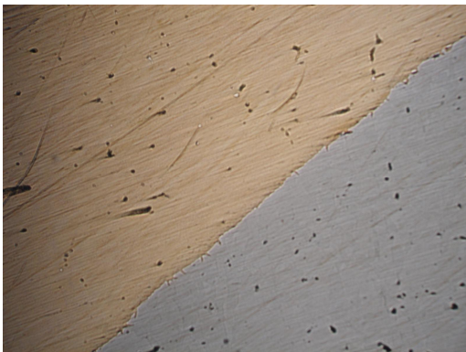
Figure 6: Aspect of bimetal at interface (100X without exposure to metallographic attack)
