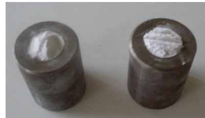
Figure 3: Preparation of the samples before introduction in the heating furnace
