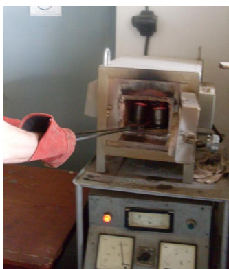
Figure 2: Furnace used to melting the bronze chips into steel support
