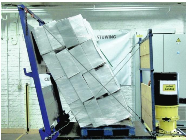
Figure 1: The acceleration test machine after an acceleration test, with a failed load unit.
